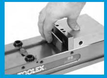
Snap in the parallels or soft jaws that you require for your setup and begin machining. Two lock screws are provided for extra holding assurance, but are not necessary to hold parallels in place. Do not overtighten lock screws.
